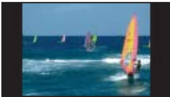
4/3 mode: Image shows a 4/3 source Places the 4/3 image in centre of the screen with black bands on either side.
