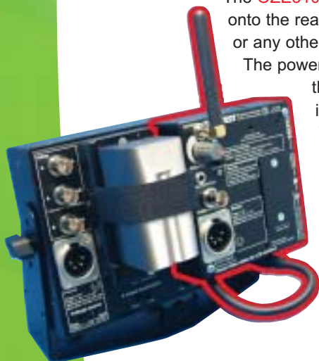
OZE3100 receiver fixed to the rear of the monitor
